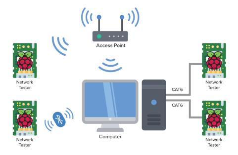
The above diagram shows how a PC with network interfaces can be tested via multiple network testers.
