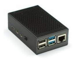
To avoid the bare Pi board accidently touching a piece of metal and shorting out, a case is needed. Furthermore, once in a case, having a heatsink and fan is necessary to keep the CPU cooler and therefore avoid throttling.
